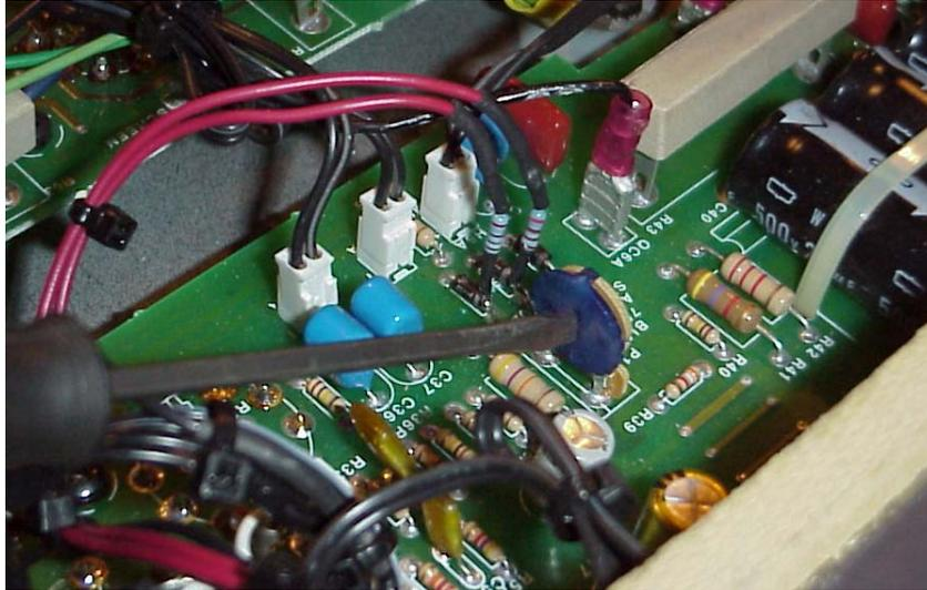
This is the bias adjust pot. Turn it towards the back of the amp to reduce current, and towards the front of the amp to increase current. Make small adjustments, you will probably find that as you get the current just where you want it, it will go too far, and small adjustments either way will be too much. Be patient, make small adjustments, and let the current stabilize. Take your time and get it just right.
