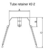
• Materials ; Steel plate with Ni plating and natural coil spring
